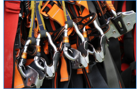
Full body harnesses are commonly used for fall protection when Passive Systems are not feasible.
